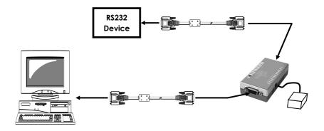
3. Connect the 5V AC Adapter or USB-to-Power-DC-Jack Conversion Cable
