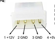
For using the EX-11087 you must connect the card with the PC power supply. Please make sure you connect the plug in the right direction.
