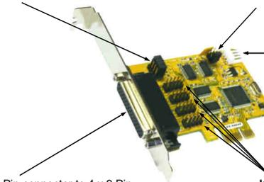
S1-S4: 44 Pin connector to 4 x 9 Pin serial connectors
