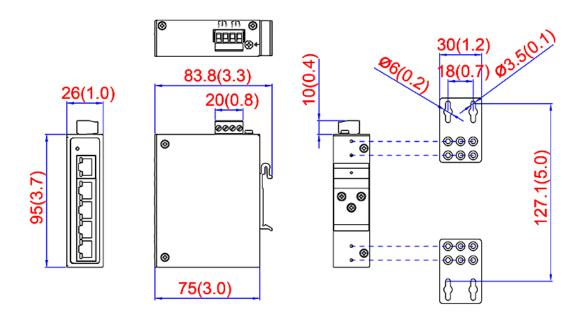
Unit: mm (inch) Din-rail Wall-mount
